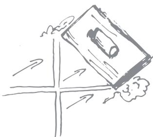
Use the float to apply the grout to the joints between the tiles. The rubber side of the float is used to press the grout into the joints. Ensure you wipe away any surplus grout from the surface of the tiles using a sponge as you go.
