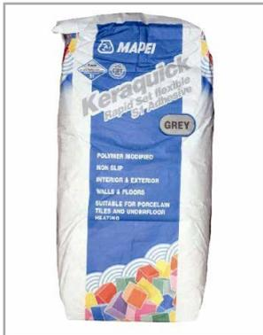
[Keraquick Grey/White](#) is a rapid setting flexible adhesive for use with ceramic, porcelain and natural stone including mosaics in wet or dry areas. Suitable for use on plywood overlay and underfloor heating systems, it has a working time of 30 mins once mixed, a coverage of approximately 5m<sup>2</sup> using a 10mm notched trowel and can be grouted after 2 hours. Remember to always use white adhesive with light coloured natural stone products such as travertine.
