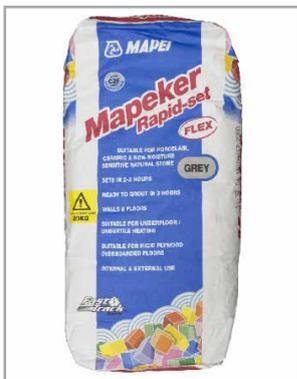
[Mapeker Rapidset Flex Grey](#) is a fast setting flexible grey adhesive suitable for ceramic, porcelain, mosaics and natural stone, (e.g. slate) in wet or dry areas. Suitable for use on concrete, sand/cement screed, plywood overlay and underfloor heating. It has a working time of 20 mins once mixed, a coverage of approximately 5m<sup>2</sup> using a 10mm notched trowel and can be grouted after 3 hours.
