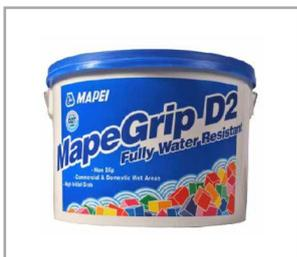
**MapeGrip D2** is a water resistant adhesive for fixing porous bodied glazed wall tiles in internal domestic or commercial installations. Suitable for use in showers. Both adhesives have coverage of approximately 6m<sup>2</sup> when using a 6mm notched trowel, and can be grouted after 24 hours.
