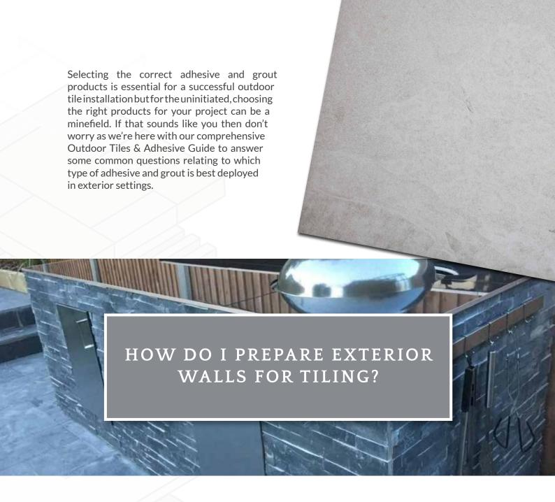
If you're tiling an exterior wall you'll first want to ensure that the substrate you're attaching the tiles to is suitable. Brick walls are fine, as are plastered ones, but you must make sure that they're level and will bear the load of the tiles you're fixing to them first. Priming is essential where absorption needs to be reduced on surfaces such as render, plywood, plaster, plasterboard and sand:cement screeds.
