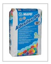
Adesilex P9 White is a slow setting non flexible adhesive suitable for ceramic, porcelain and mosaics in wet or dry areas (not suitable for swimming pools). Suitable for use on plaster, plasterboard, render concrete, sand cement screed and tile backer boards. It has a working time of 8 hours once mixed, a coverage of approximately 5m2 using a 10mm notched trowel and can be grouted after 24 hours.
