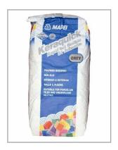
Keraquick Grey/White is a rapid setting flexible adhesive for use with ceramic, porcelain and natural stone including mosaics in wet or dry areas. Suitable for use on plywood overlay and underfloor heating systems, it has a working time of 30 mins once mixed, a coverage of approximately 5m2 using a 10mm notched trowel and can be grouted after 2 hours. Remember to always use white adhesive with light coloured natural stone products such as travertine.
