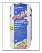
Mapeker Rapidset Flex Grey is a fast setting flexible grey adhesive suitable for ceramic, porcelain, mosaics and natural stone, (e.g. slate) in wet or dry areas. Suitable for use on concrete, sand/cement screed, plywood overlay and underfloor heating. It has a working time of 20 mins once mixed, a coverage of approximately 5m2 using a 10mm notched trowel and can be grouted after 3 hours.
