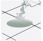
Ensure surface to be treated is clean and as dry as possible before pouring the sealer onto the surface.
