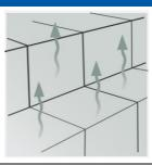
STEP 3. Leave the solution to penetrate the surface. Leave for 1 – 5 hours depending on the level of soiling.
