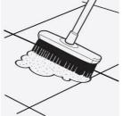
Grout in the joints or brush in jointing compound and clean off residues. Always follow manufacturers instructions.
