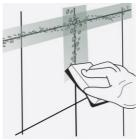
Apply to the surface of the grout joints using a sponge soaked in the solution.
