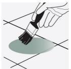
STEP 2. Spread out evenly using a paint brush and leave for 30 - 40 minutes.
