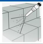
STEP 5. Rinse well with plenty of water. Allow surfaces to dry before allowing traffic or sealing applying porcelain protector.
