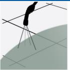
STEP 2. Wet the surface with the solution and leave for 10 – 15 minutes. Work in manageable areas at a time.
