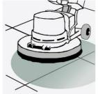
STEP 3. Scrub surfaces with a rotary scrubber to release cement & salt residues.
