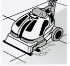
STEP 3. Set solution release rate on the machine and scrub surfaces.
