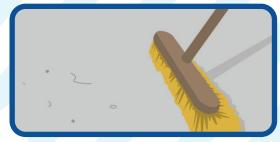
Brush surface clear of any loose dirt and debris, Prime with **Norcros Prime Bond.**
