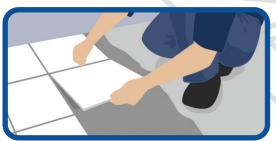
Apply **Norcros Rapid Porcelain Tile Adhesive** using a suitable notched trowel. Tile as normal.
